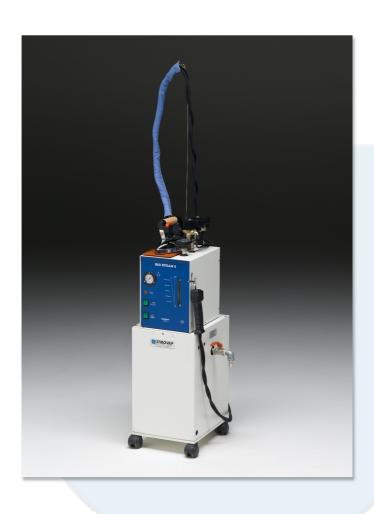
industrial steam generator with round boiler 5 Liters, pressure switch for exact control of steam pressure, visual control of the waterline in the boiler, ball valve for deposit and water outlet, steam valve with control of steam flow, safety valve cap, No. 02 safety thermostats to protect the heating elements in case of lack of water and to protect the boiler against too high temperatures and it is supplied complete with and industrial steam iron.
