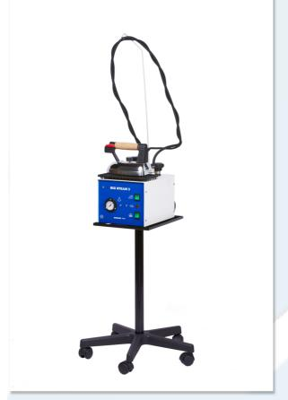
industrial steam generator with round boiler 3 Liters, pressure switch for exact control of steam pressure, steam valve with control of steam flow, safety valve cap, No. 02 safety thermostats to protect the heating elements in case of lack of water and to protect the boiler against too high temperatures, acustic alarm for lack of water in the boiler.
